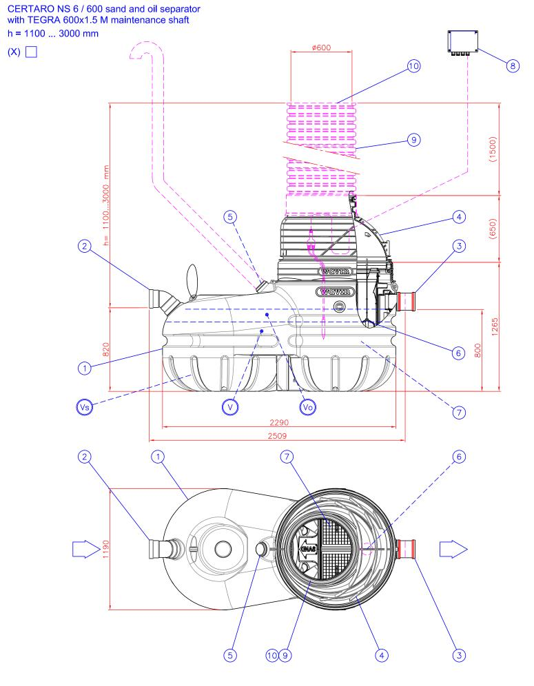
h = Installation heigth from inlet to ground surface
