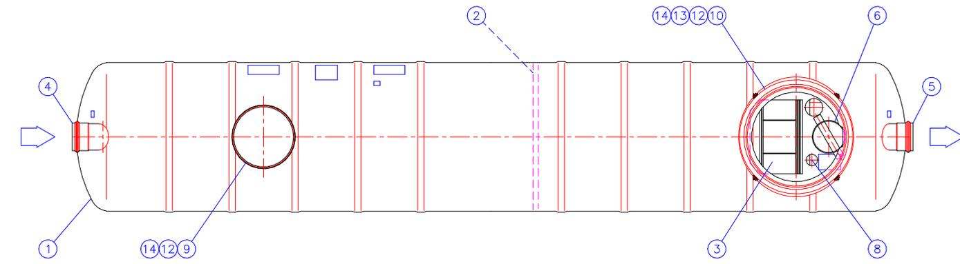
**NOTE! SPECIAL MODEL. Oil separator class I (EN858) integrated with sand trap (Vol. 6000 l). Separator with automatic closure device (DN250).**
