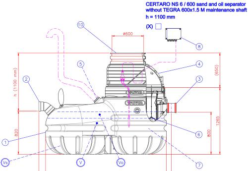
Maximum SLW60 (100kN/m²) traffic load if 1,0m hard surface coverage above inlet (water level). Maximum groundwater level 2,5m above bottom of tank. Maximum depth is 3,0m from cover down to inlet (water level).
