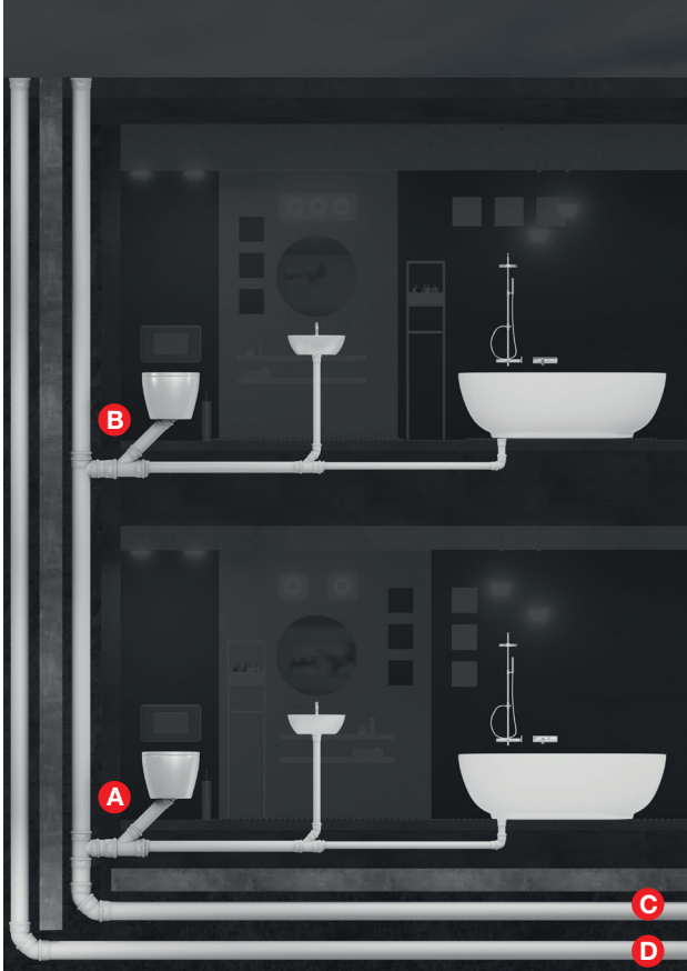
Fig. 11: Minimum fall for waste water pipes, example.
