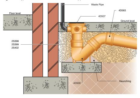
Figure 13: Typical waste pipe connection to Bottle Gully
