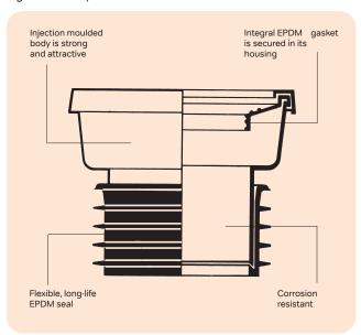
Figure 24: Connection to ground floor WC
