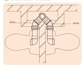
Figure 27: Alternative back-to-back WC installation
