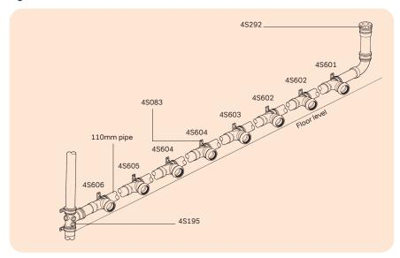
Figure 30: Typical layout of double manifold float
