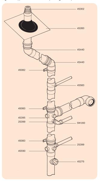
Figure 2: Typical stack assembly – Solvent Weld system
