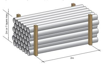
Figure 40: Storage of loose pipe on bearers
