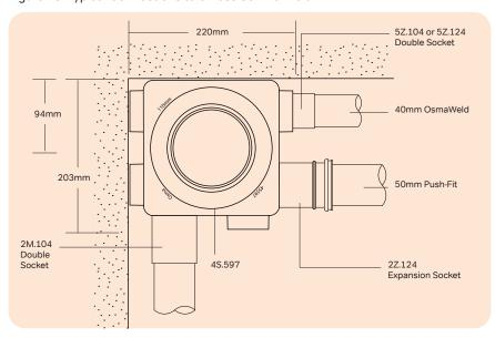
Figure 19: Typical Bathroom Installation using 6 Boss Soil Manifold 4S597
