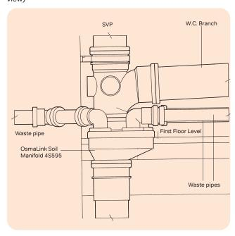
Figure 62: Typical OsmaLink Soil Manifold installation (plan view)
