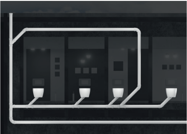
Fig. 23: Air-circulation pipe.
