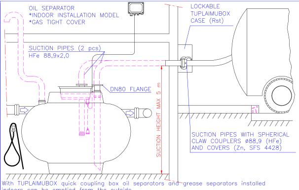
indoors can be emptied from the outside. TUPLAIMUBOX is made of stainless steel and includes 2 pcs spherical Ø88,9 claw couplers (HFe, SFS 4428) and also 2 pcs Zn-covers. On the inner surface of the hinged cover are instructions for emptying the separator.
