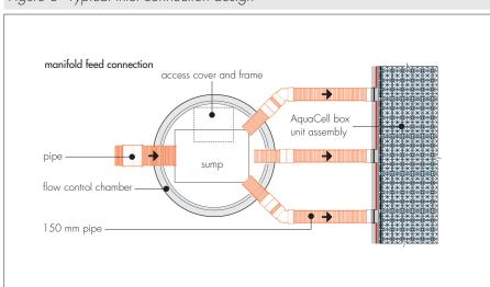
Figure 3 Typical inlet connection design
