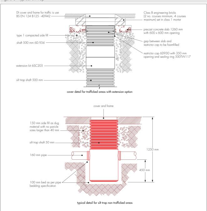
11.5 For all flow control devices it is sensible to incorporate access (via a manhole or similar) to the location of the pipe entry, orifice or vortex valve. This will enable easy removal of any blockage. The orifice itself may be protected by a debris screen.
