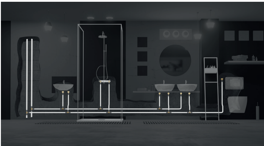
Fig. 42: Single Tee installation.
