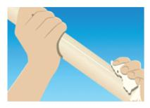
b) Cut the pipes squarely using recommended cutters or a hacksaw. Remove debris with the aid of a blade, making sure that the surface is smooth. The surface must not be sanded.
