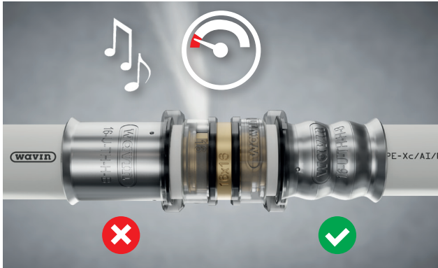
Fig. 33: Acoustic Leak Alert when testing with air.
