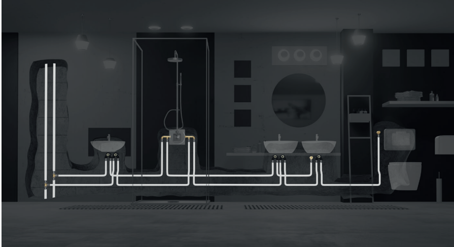
Fig. 43: In series installation.
