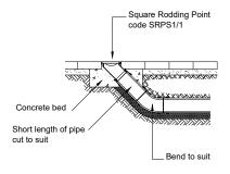
Max depth – n/a Loading 35 kn (1 tonne wheel load) Airtight Screwed down cover
