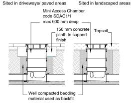
Max depth – 0.6 metres Loading 35 kN (1 tonne wheel load) Airtight Screwed down cover Main channel – 100 mm Side inlets – 2 no 100 mm at 45 °
