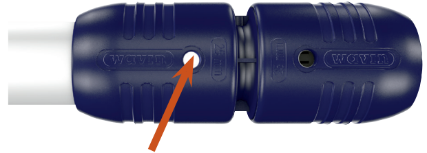
Figure 8: The observation window in the PPSU cap can be used to check that the pipe is inserted to the stop.
