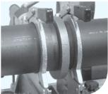
11. Maintain heat soaking until a bead is formed of approximate 1mm for diameters 40 up to 200 and 1.5mm for diameters 250 and 315mm. Use the figures mentioned in table 2 as guidance for the
