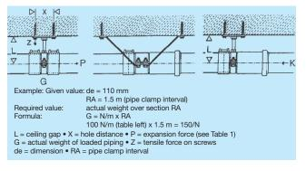
Reduction collars can be used to achieve the required diameters. Fixings used must be capable of withstanding the actual weight of the loaded piping and the resulting tensile forces generated
