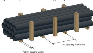
Figure 16: Pipes stored on timber supporting frame
