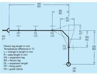
Figure 1: Installation using flexion legs
