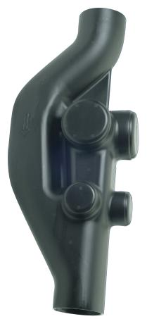
The Wavin HDPE Airmix "Sovent" fitting prevents all this. The principle of this fitting is based on keeping a free path air to leave or to enter the system and thereby keeping the pressure level within acceptable limit.
