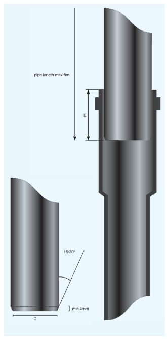
induced displacements, expansion joints can be positioned in horizontal collector pipes.
