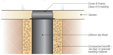
Figure 13: Installation detail A15 – For non-driveway applications subject to infrequent vehicle loading up to 15kN (1.5 tonnes)
