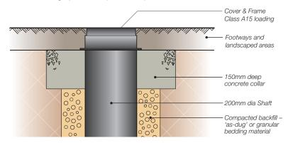
For both non-load and infrequent loading applications, as above
