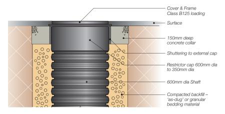
Figure 24: Installation detail for B125 loading: paved areas with limited traffic load
