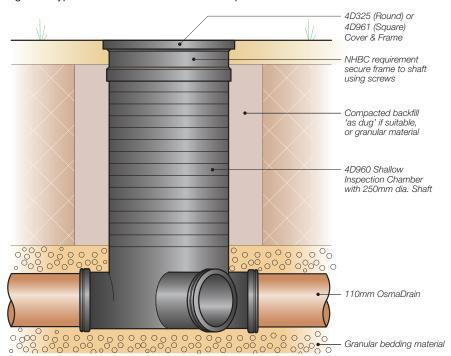
Figure 2: Typical installation detail: Multi-Base Inspection Chamber
