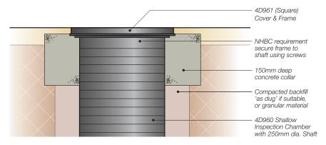
Figure 5: Installation detail - green areas (non-loaded)
