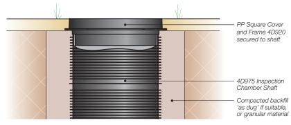
Figure 9: Installation detail Class A15 – areas subject to occasional vehicle loading up to 15kN (up to 5 tonnes when supported with a concrete plinth). For heavier vehicles (ie. Electric vehicles, 4x4s, pick-up trucks & vans), B125 cover should be used
