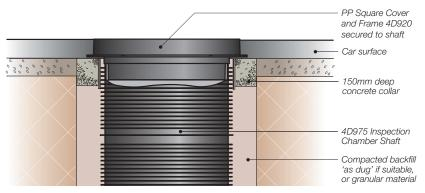
4D920 up to 5 tonnes when supported with a concrete plinth
