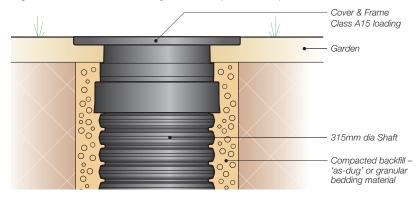
Figure 17: Installation detail A15 – For non-driveway applications subject to infrequent vehicle loading up to 15kN (1.5 tonnes)
