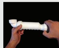
3- Rotate and connect the HepvO Anti-Odor valve outlet side and union thread to the valve. Check for proper installation by pulling the below hose.
