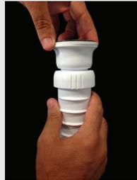
4- Connect the sink strainer to the upper union inlet part of the HepvO diaphragm by rotating it clockwise. Torque the gasket by tightening the union. The gasket that comes with the kit for d32 HepvO connection must be used separately.
