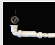
5- In order to connect it to the sink, remove the screw on top of the strainer and connect it so that the sink remains in between the metal strainer and the plastic base.
