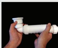
4- Connect the sink strainer to the upper union inlet part of the elbow by rotating it clockwise. Torque the gasket by tightening the union. The gasket that comes with the kit for d32 HepvO connection must be used separately.
