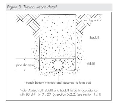
15.1 Where the as-dug material is suitable<sup>(1)</sup> for use as bedding, the bottom of the trench may be trimmed to form the pipe bed.
