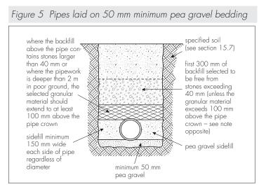
15.8 When the 150 mm pipes are to be laid on rock, compacted sand or gravel requiring mechanical means of trimming, or in very soft or wet ground, the bedding should be as detailed in section 15.5.
