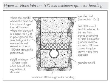
15.6 The trench formation should be prepared, the bedding placed and the pipes laid in accordance with BS EN 1610 : 2015, BS 8000-0 : 2014 and BS 8000-14 : 1989.
