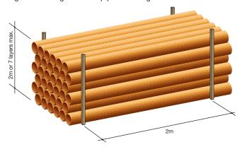
Figure 4: Storage of loose pipes on bearers
