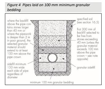
16.6 The trench formation should be prepared, the bedding placed and the pipes laid in accordance with BS EN 1610 : 2015, BS 8000-0 : 2014 and 8000-14 : 1989.
