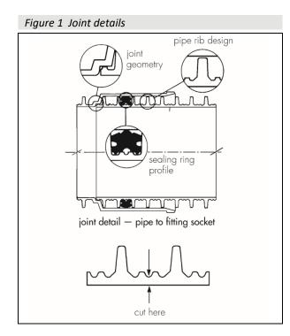
15.1 The pipes are cut midway between the ribs, as shown in Figure 1.
