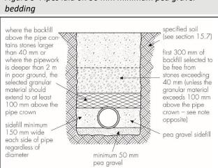
Figure 5 Pipes laid on 50 mm minimum pea gravel
