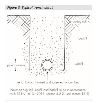
16.1 Where the as-dug material is suitable<sup>(1)</sup> for use as bedding, the bottom of the trench may be trimmed to form the pipe bed.
