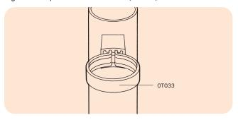
Figure 43: Use of Pipe Bracket Spacer
