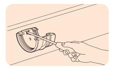
Figure 27: Installation of RoundLine Gutter Union
