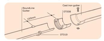
Figure 29: Connection to cast iron gutter
