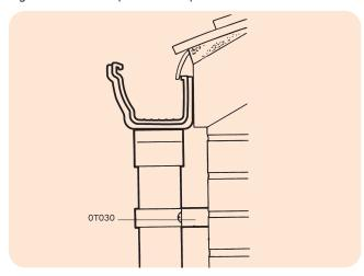
Figure 44: Application of Pipe Bracket Spacer
