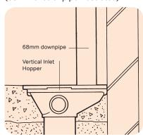
Figure 18: Connection to bottle gully
