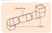
Plain ended 68mm circular and 61mm square pipe connects directly to the sockets of the Running Outlet 8T806 and the Stopend Outlets 8T807/808.
