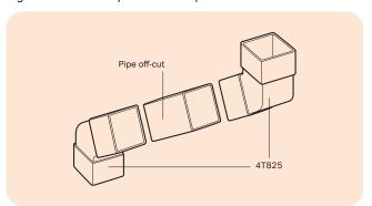
Figure 46: RoofLine shallow offset
