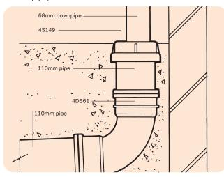
Figure 49: Connection to 110mm PVC-U Socket (61mm square pipe)
