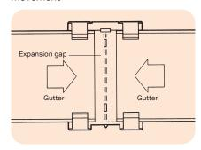
A gutter jointing bracket or gutter union with bracket should be fitted within 300mm from the end of terminal lengths of gutter.
