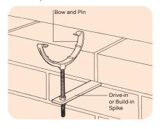
Figure 34: Installation of Rise and Fall Brackets
