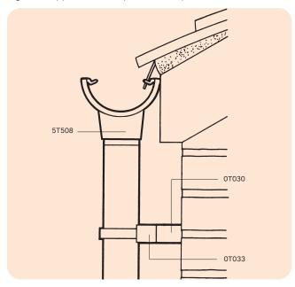
Figure 9: Use of Pipe Bracket Spacer
