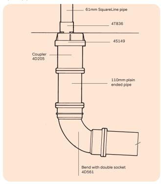
Figure 50: Connection to 110mm PVC-U Socket (61mm square pipe)
