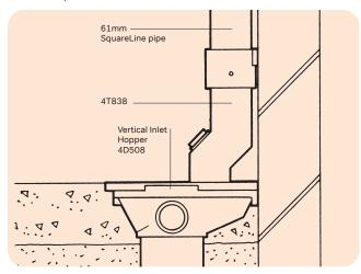
Figure 57: 110mm Connection to PVC-U Drain Socket
