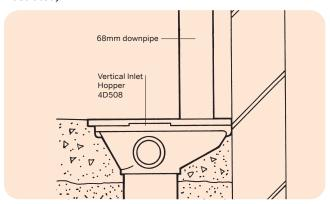
Figure 56: Connection to Bottle Gully (61mm square pipe illustrated)
