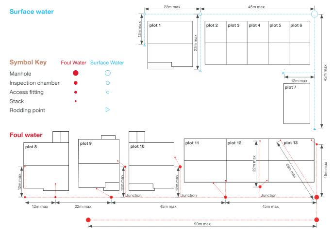
This drawing is to illustrate the recommended maximum spacing of access provision (in metres) for manual cleaning only. Diagrammatic only - not to scale.
