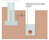
When D is 1m or more, concrete fill to within D-150mm of level of foundation bottom.
