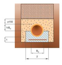
b. Reinforced concrete bed. Bedding factor 3.4 (0.4% steel)
