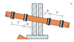
a. Pipe built-in to structure
