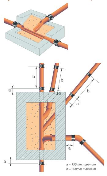
Fig. 38 – Branch channel bend selector (for half section and 3/4 section)
