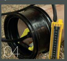
Apply pressure to achieve a 110mm water gauge on the manometer
