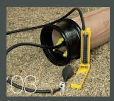
Connect a "U tube" gauge (manometer) to the testing stopper
