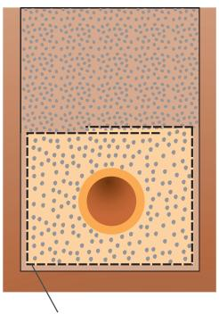
Geotextile wrapped over pipe bedding/surround
