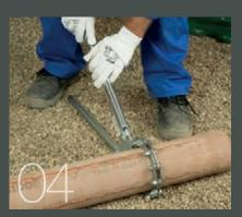
Tighten the chain, by pulling the arms together
