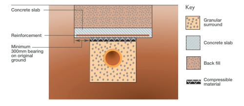
Laying vitrified clay pipes on recycled material (TN7)
