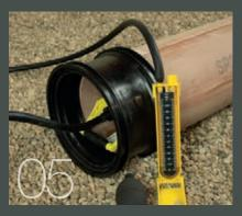
Allow approx. 5 minutes for stabilisation before adjusting the pressure to 100mm water gauge.
