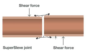
Note that differential movement can occur when pipes enter buildings or connect with an inspection chamber, manhole, wall or other structure.
