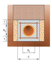
c. Reinforced concrete surround. Bedding factor 4.8 (4  $\times$  1% steel). Reference: TRRL Simplified tables [2]
