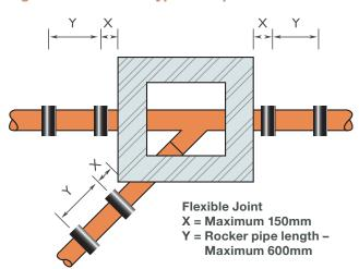
Fig. 9 – Diagrammatic sections showing pipes passing through walls
