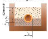
Granular bed and haunch. Generally suitable for all soil conditions.
