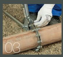
Hook the chain onto the jaw of the pipe cutter
