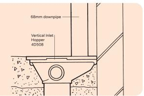
Figure 56: Connection to Bottle Gully (61mm square pipe illustrated)
