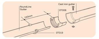
Figure 29: Connection to cast iron gutter
