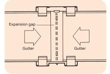
A gutter jointing bracket or gutter union with bracket should be fitted within 300mm from the end of terminal lengths of gutter.
