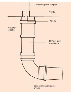
Figure 50: Connection to 110mm PVC-U Socket (61mm square pipe)
