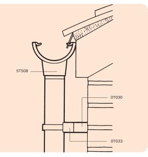
Figure 9: Use of Pipe Bracket Spacer
