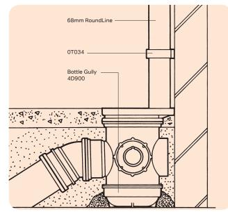
Figure 55: Connection to Bottle Gully (68mm Circular pipe illustrated)
