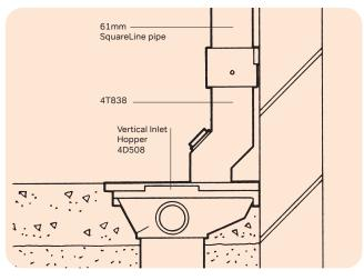
Figure 57: 110mm Connection to PVC-U Drain Socket
