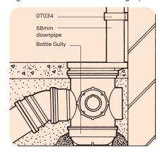
Table 10: Connections to Below Ground Drainage
