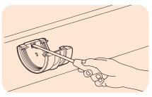
Figure 27: Installation of RoundLine Gutter Union
