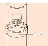
Figure 43: Use of Pipe Bracket Spacer
