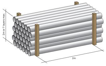
Figure 22: Storage of loose pipe on bearers
