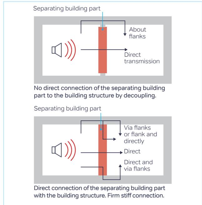
Figure 7: Information on the possible transmission paths for different building parts
