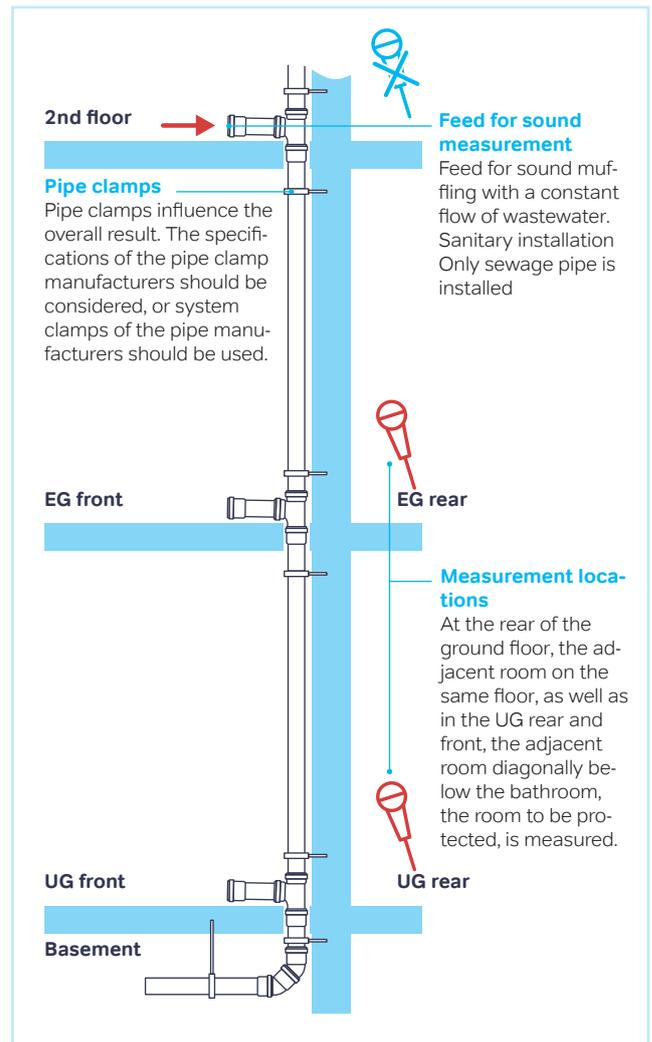
**Figure 45:** Measurement setup according to DIN EN 14366
