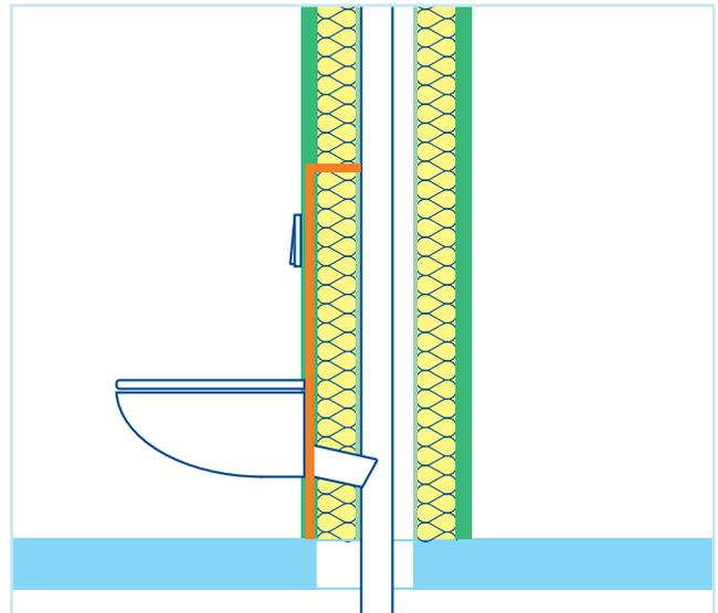
Figure 33: In-wall installation (based on source 8)
