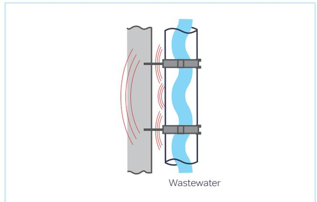
Figure 16: Structure-borne sound
