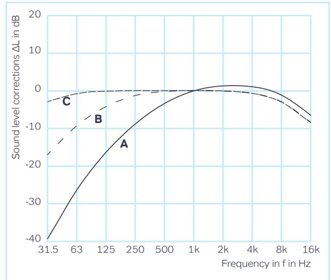
Figure 2: Sound pressure level correction  $\Delta L$  according to DIN EN ISO 16032 (or the withdrawn DIN EN 60651) for ratings A, B, and C
