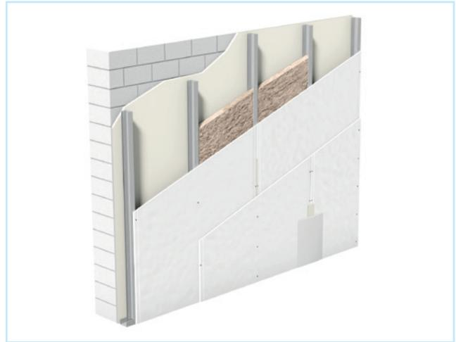
**Figure 24:** Advance wall construction in front of a solid wall (source: Knauf)
