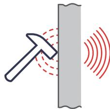
⌚ **Structure-borne sound** originates in solid bodies and propagates at the surface as airborne sound. In pipe installations, this happens mostly through pipe clamps and brackets in the wall.
