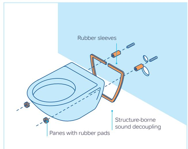
**Figure 26:** Design of a wall hung toilet system without sound bridges
