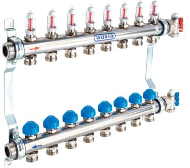
The stainless steel blending manifolds are used for distributing and regulating the volume of flow in low temperature floor heating or cooling systems. This manifold blends and reduces the water temperature from the heat source to the correct operating temperature for the underfloor heating, The pump manifold utilises a Grundfos UPM3. The maximum permissible continuous operating pressure is 5 bar at 80°C. The maximum permissible test pressure is 10 bar at 20°C.
