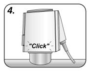
The Wavin Comfia Actuator snaps onto the valve adapter with a "click" when pressed down vertically by hand.
