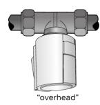
The Wavin Comfia Actuator must be installed preferably in vertical or horizontal installation position. In case of "overhead" installation, special circumstances (e.g. drainwater) can reduce the lifetime of the actuator.
