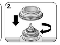
Screw the valve adapter manually on the valve.
