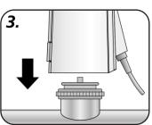
Place the Wavin Comfia Actuator vertically on the valve adapter.
