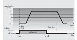
In case of the normally closed version, the valve is opened steadily by the ram motion upon switching on the operating voltage and after expiry of the dead time.
