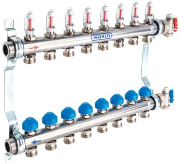
The stainless steel blending manifolds are used for distributing and regulating the volume of flow in low temperature floor heating or cooling systems. This manifold blends and reduces the water temperature from the heat source to the correct operating temperature for the underfloor heating, The pump manifold utilises a Grundfos UPM3. The maximum permissible continuous operating pressure is 5 bar at 80 °C. The maximum permissible test pressure is 10 bar at 20 °C.
