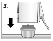
Place the Wavin Comfia Actuator vertically on the valve adapter.
