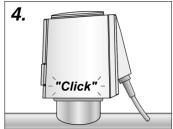
The Wavin Comfia Actuator snaps onto the valve adapter with a "click" when pressed down vertically by hand.
