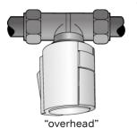
The Wavin Comfia Actuator must be installed preferably in vertical or horizontal installation position. In case of "overhead" installation, special circumstances (e.g. drainwater) can reduce the lifetime of the actuator.
