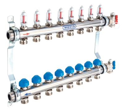
The stainless steel standard manifolds are used for distributing and regulating the volume of flow in low temperature floor heating or cooling systems. This manifold is suitable for use in systems where the main heat source is providing water at the correct operating temperature for the underfloor heating. The maximum permissible continuous operating pressure is 5 bar at 80 °C. The maximum permissible test pressure is 10 bar at 20 °C.
