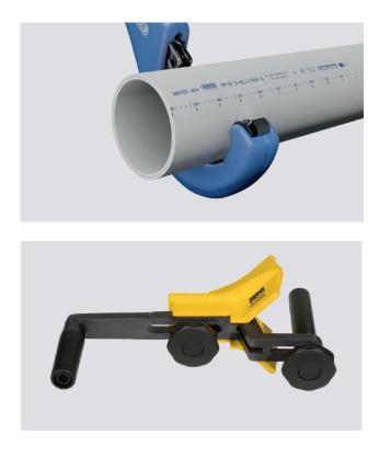
For connections to Wavin AS+ fittings or sockets the pipe end needs to be chamfered. Its is recommended to chamfer over a length of 5 mm under a 15 degrees angle. This can be done by using standard chamfer tooling.
