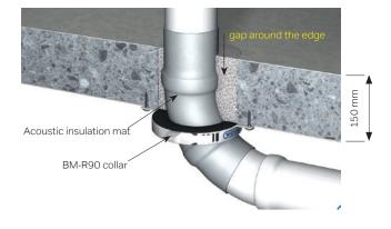
Fig. 44: Straight installation with / without sleeve / socket.
