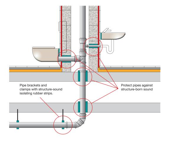
Fig. 9: Sound insulation of waste water systems.
