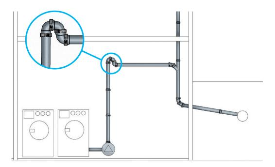
Fig. 30: Tensile resistant connection.
