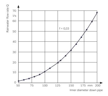
Fig.: 25: Drainage performance of rainwater downpipes.
