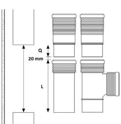
When replacing a piece of pipe, secure that the total length of the new socketed pipe (L) equals the length of the part cut out minus the length of the spigot of the branch (Q) minus 20 mm.
