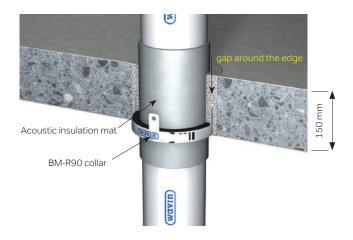
Fig. 40: Straight installation with / without sleeve / socket.
