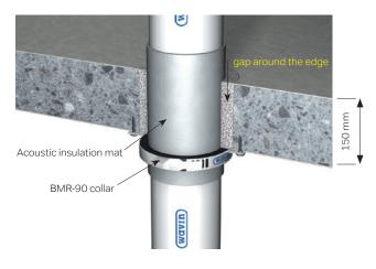
Fig. 43: Straight installation without sleeve / socket up to 160 mm.
