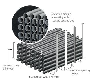
Stack pipes of different sizes separately or, if this is not possible, stack them in such a way that the largest diameter pipes are at the bottom. Pipes with sleeves should be stacked alternately so that they are supported along their entire length (see picture). Fittings are supplied in boxes and must be stored indoors. Do not subject fittings to heavy loads, as this can deform them.
