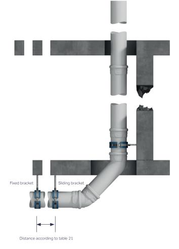
Fig 36: Example horizontal and vertical installation.
