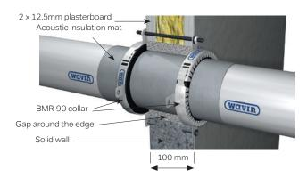
Fig. 47: Straight installation without sleeve / socket.
