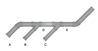
Fig. 21: Example collector pipe with primary ventilation.
