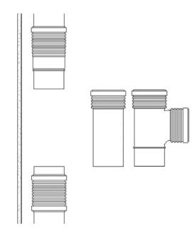
**7.** Push the socketed of the branch or pipe on to the long socket.
