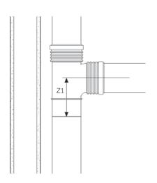
Install a short piece of temporary pipe halfway onto the repair coupler to secure a correct positioning of the rubber seal. **3.** Install the free half of the coupler onto the existing pipe and slide the repair coupler completely over the existing pipe.
