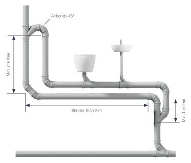
Fig. 23: Bypass pipe conforming to DIN 1986-100.
