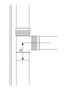
When inserting a branch, the length of the part to be cut out should have the length of the branch (L) + 20 mm + the length of the spigot of the long socket (Q).
