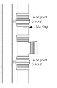
When inserting a branch at a later stage, please secure that the level of the branch is located at the right height. The Z1 value is mentioned for each branch in the product overview.
