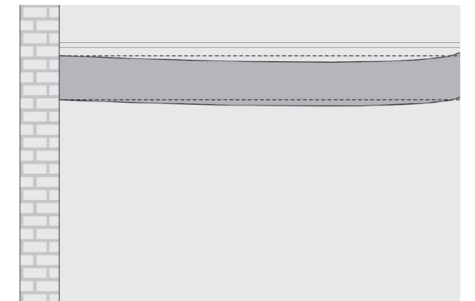
Figure 28: Water accumulation may cause bending of the roof
