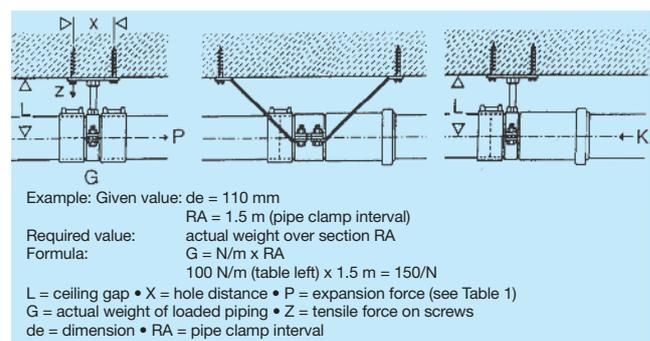
Reduction collars can be used to achieve the required diameters. Fixings used must be capable of withstanding the actual weight of the loaded piping and the resulting tensile forces generated
