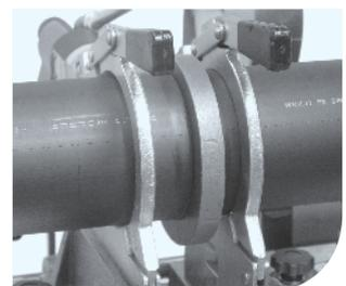
11. Maintain heat soaking until a bead is formed of approximate 1mm for diameters 40 up to 200 and 1.5mm for diameters 250 and 315mm.
