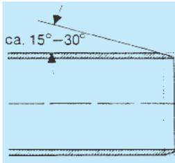
Figure 4: Fixing a long pipe collar
