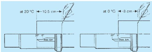
Pipe ends should be evenly chamfered to an angle of approximately 15°. Use silicone lubricant on the spigot end as this allows the pipe end to be inserted with minimum resistance.
