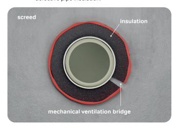
Wavin Hot and Cold Water Systems already laid on the floor are exposed to many potential impacts on site during the construction phase, from scaffolding, ladders or other objects. Therefore caution must be exercised to prevent damage to the pipe/fitting or even the insulation. Before installing further floor construction, a check should therefore be conducted for damage. Any damage to the pipe insulation should be
