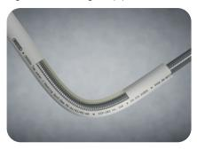
By bending the pipe the demand of fittings needed for the installation can be reduced. The pipe is easy to bend: by hand, with the aid of the bending spring or using the Wavin bending pliers. Bending springs and bending pliers are preferred to be used to ensure the pipe is not kinked by accident. Larger diameters can be bend with pliers with appropriate dimensions, bending radius min. 3xDa.
