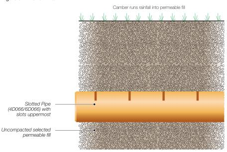
Figure 38: Bedding of slotted pipes for disposal of septic tank effluent
