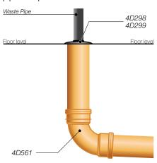
Figure 15: Internal connection of 110mm diameter soil pipe
