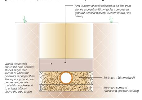
Figure 6: OsmaDrain pipes laid on 100mm minimum of processed granular material
