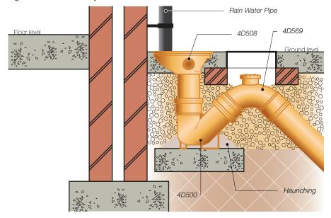
Figure 28: Universal Gully - protection of outlet bend
