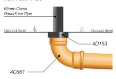
Figure 21: Connection of SquareLine Rainwater Pipes
