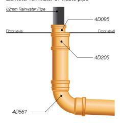
Figure 17: Connection of RoundLine rainwater pipe to OsmaDrain 110mm spigot
