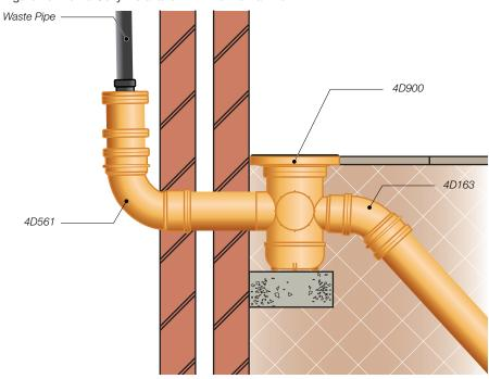
Figure 30: Bottle Gully installation with vertical inlet
