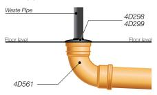
Figure 14: Connection of internal waste pipe at depth
