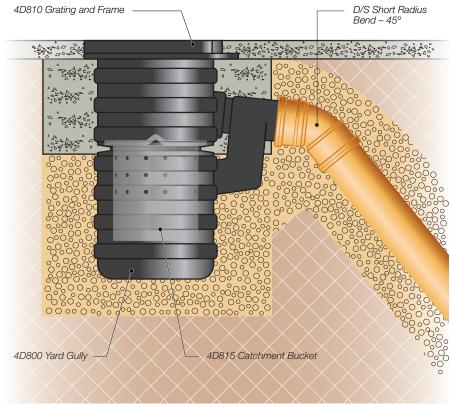
Figure 33: Yard Gully installation
