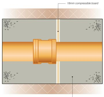
150mm concrete surround of suitable strength placed in one operation (Reinforced if necessary)
