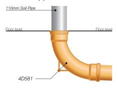
Figure 16: Internal connection of 82mm diameter rainwater or waste pipe
