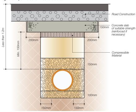
Figure 9: Pipe Protection – concrete surround
