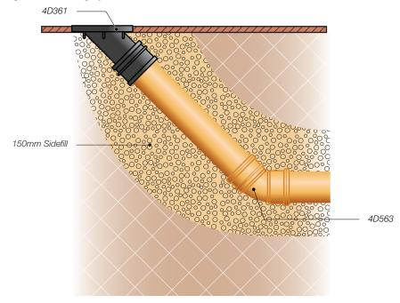
Figure 26: Rodding Eye - intermediate access
