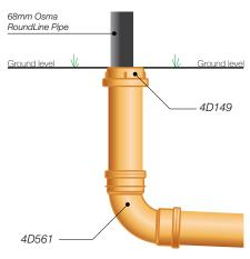
Figure 18: Connection of RoundLine rainwater pipe to OsmaDrain 110mm socket
