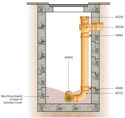
Figure 23: Open Channel Manhole with stepped invert and external backdrop
