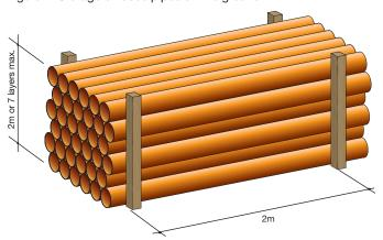
Figure 3: Storage of loose pipes on bearers
