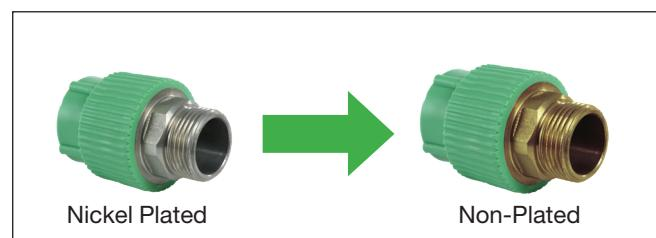
The new PPR Fittings are non-coated brass alloy which is in the acceptable alloy list in 8th revision of 4MS 2017. Metal deactivators are used in the recipe in order to avoid any damage on plastic parts that may be caused by free metal ions from inserts. This application is valid for every color of fitting. PPR Fittings will continue to meet all performance requirements of EN ISO 15874-3 standard. You can reach to international product certifications via Wavin representative.
