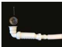
5- In order to connect it to the sink, remove the screw on top of the strainer and connect it so that the sink remains in between the metal strainer and the plastic base.
