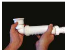
4- Connect the sink strainer to the upper union inlet port of the elbow by rotating it clockwise. Torque the gasket by tightening the union. The gasket that comes with the kit for d32 HepVO ® connection must be used separately.
