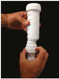
3- Rotate the union thread and attach to the valve. Check for proper installation by pulling the below hose.
