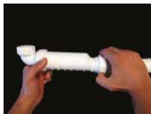
3- Rotate and connect the HepVO ® Anti-Odor valve outlet side and union thread to the valve. Check for proper installation by pulling the below hose.
