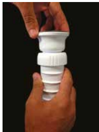
4- Connect the sink strainer to the upper union inlet port of the HepVO diaphragm by rotating it clockwise. Torque the gasket by tightening the union. The gasket that comes with the kit for d32 HepVO ® connection must be used separately.
