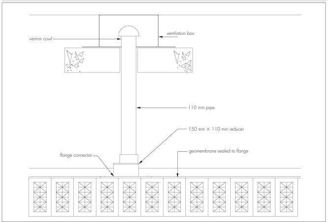
Figure 4 Typical air vent system
