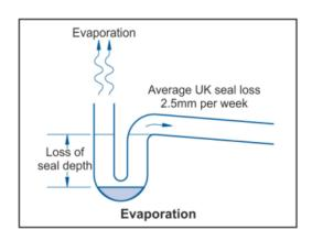
If an appliance is not used for an extended period, evaporation of the water in a traditional water seal trap will lead to a loss of the water seal. In hot climates, with higher risk of rapid water evaporation, this can be a particular problem, which can lead to odours escaping into the buildings after a relatively short period of time.
