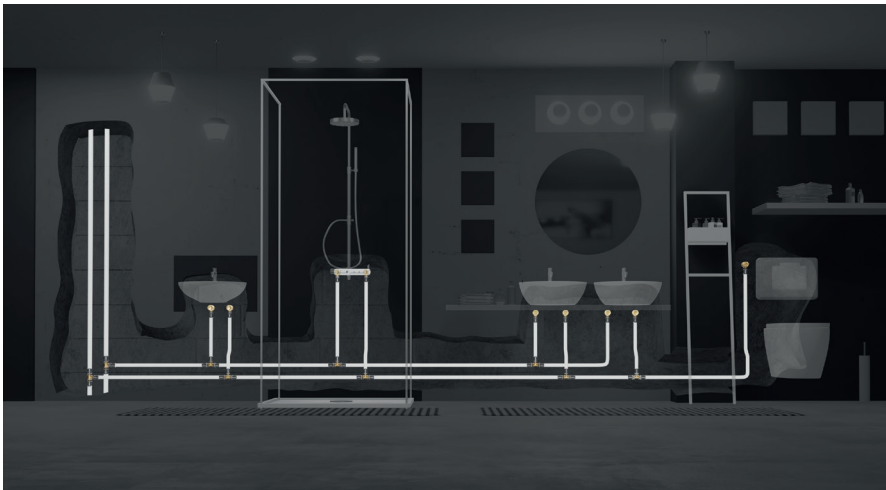
Fig. 42: Single Tee installation.
