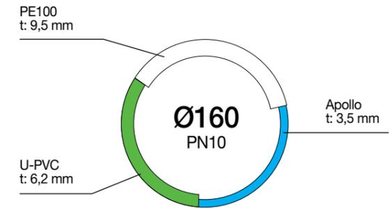
Apollo O-PVC pipes are 40-50% thinner than U-PVC pipes and 60-70% thinner than HDPE100 pipes.
