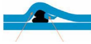
The flexible EPDM rubber seal provides sealing.
