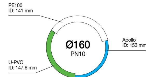
The inner diameter of Apollo O-PVC pipes is 4-7% wider than U-PVC pipes and 9-12% wider than HDPE100 pipes.
