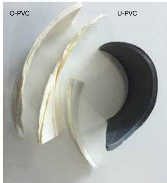
The laminar molecular structure of Apollo O-PVC pipes and the random molecular structure of U-PVC pipes can be seen through the cross section.
