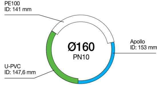
The flow area of Apollo O-PVC pipe is 7-15% higher than U-PVC pipes and 15-30% higher than HDPE100 pipes.
