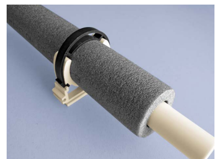
For hot water, the clip must be one size larger than the pipe (needs to be fitted over the insulation).
