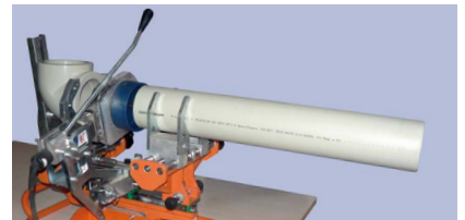
fixing and aligning the components, then heating them up
