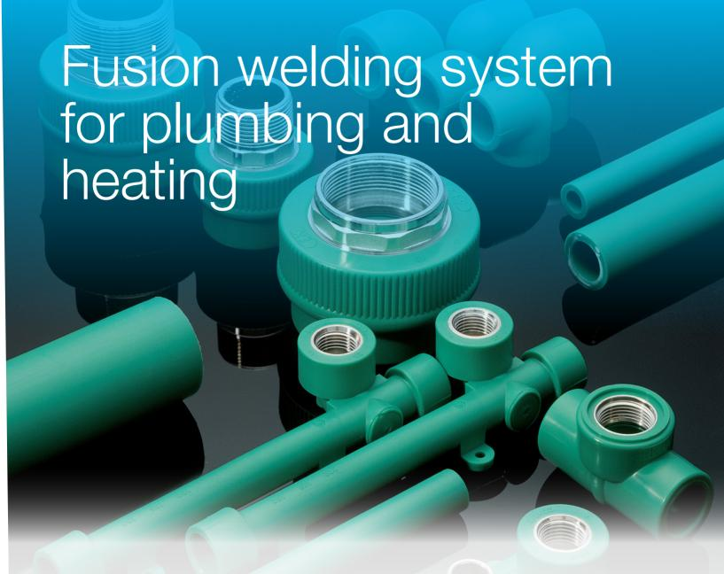
Wavin PPR is a hot and cold water supply system suitable for sanitary and potable water applications and heating systems. The pipes and injection moulded fittings are made of Polypropylene Random (PPR) type 3, also with new high performance pipes in PP-RCT (PP type 4). They are jointed by fusion welding, ensuring a homogeneous, all plastic system.
