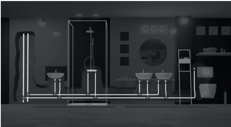
Fig. 42: Single Tee installation.
