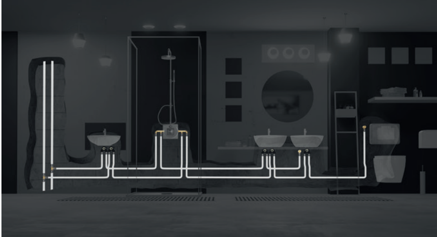
Fig. 43: In series installation.
