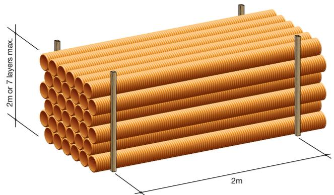
Figure 4: Storage of loose pipes on bearers
